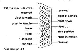
Figure 2-6. Remote Control Connector Pin Configuration
