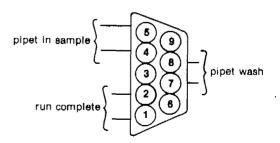
Figure 2-8. Control Sequencer Output Signals
