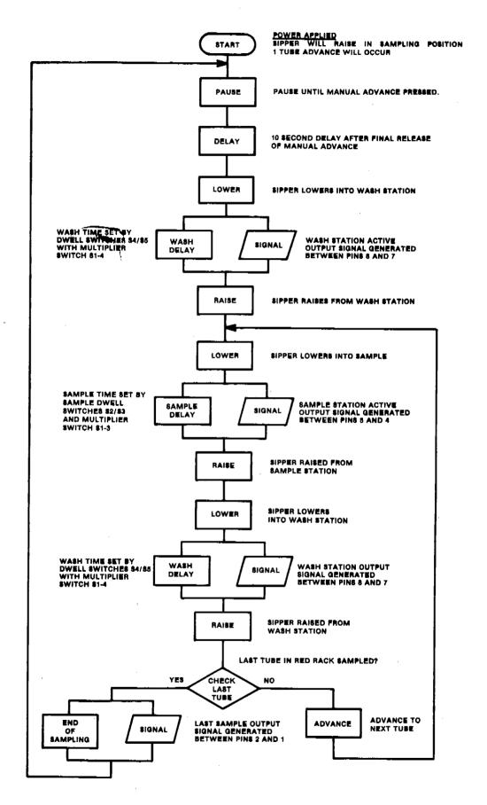
Figure 3-1. Sequence for the Autosampler with Sequencer and Wash Station
