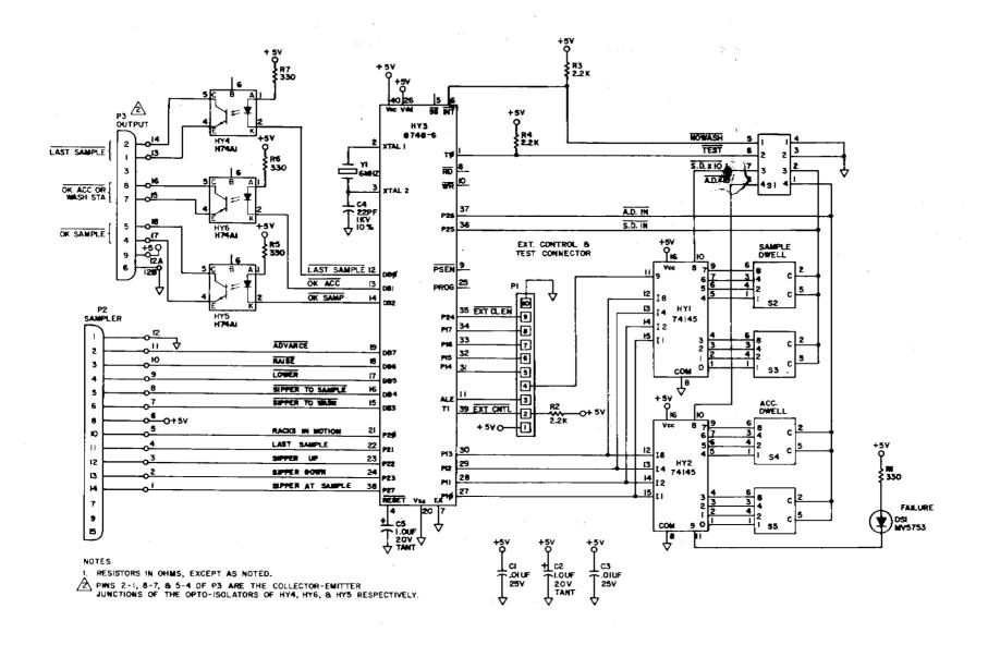
Figure 4-2. Control Sequencer Schematic
