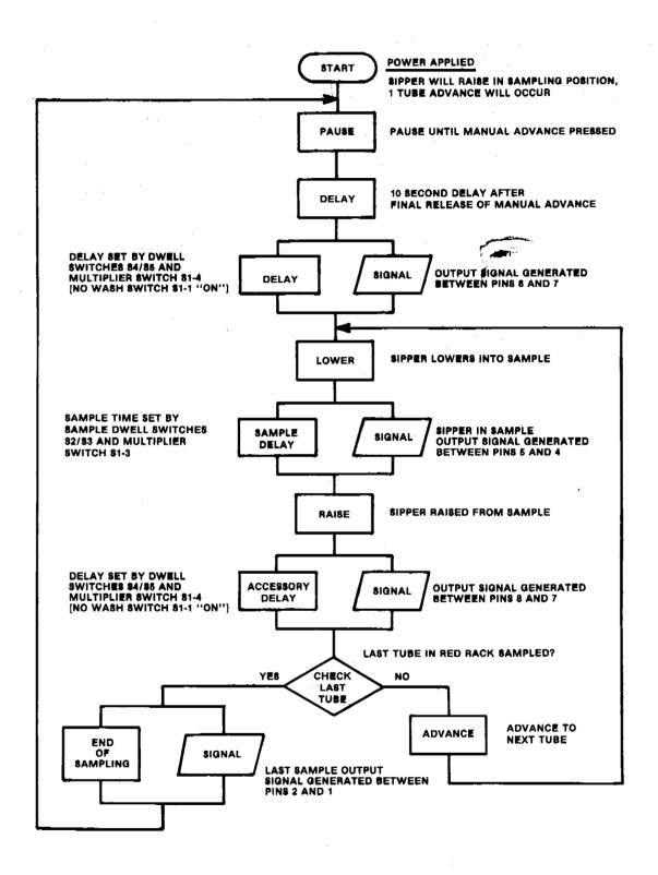
Figure 3-2. Sequence for the Autosampler with Sequencer and without Wash Station
