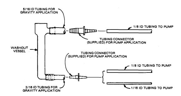
Figure 5-6. Wash Vessel Tubing Installation
